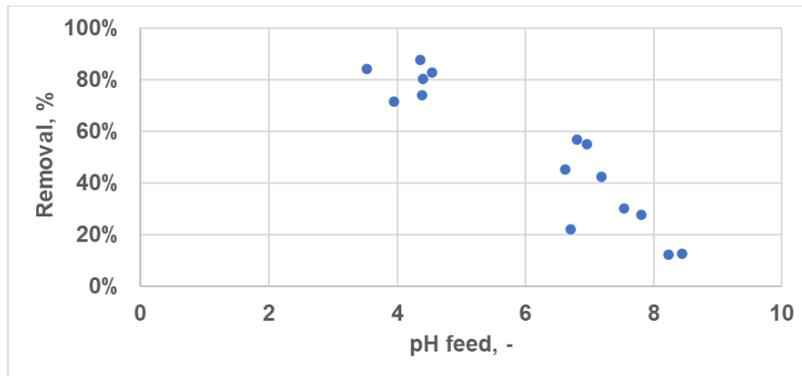
While analyzing other variables the pilot recorded (such as pH), it was possible to observe that only when the pH of the effluent (feed) is equal or lower than 4, higher removals were obtained. This allows us to also conclude that our pilot is being efficient if we control this parameter.
