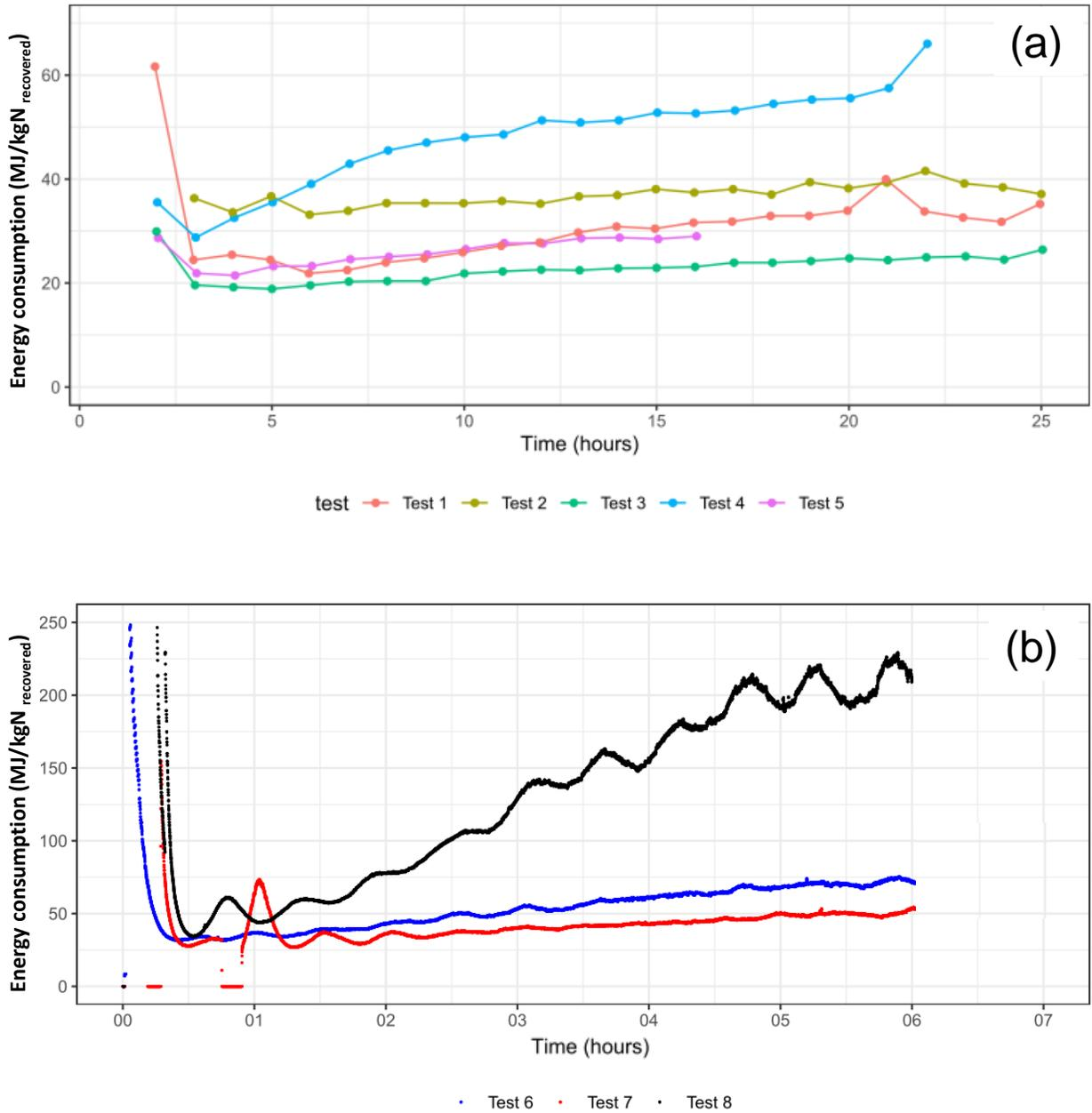
**Figure 7.** Average energy demand per hour per kg of nitrogen recovered for the experiments run in Donnan mode (a) energy demand per kg of nitrogen recovered for the experiments run in continuous mode (b).
