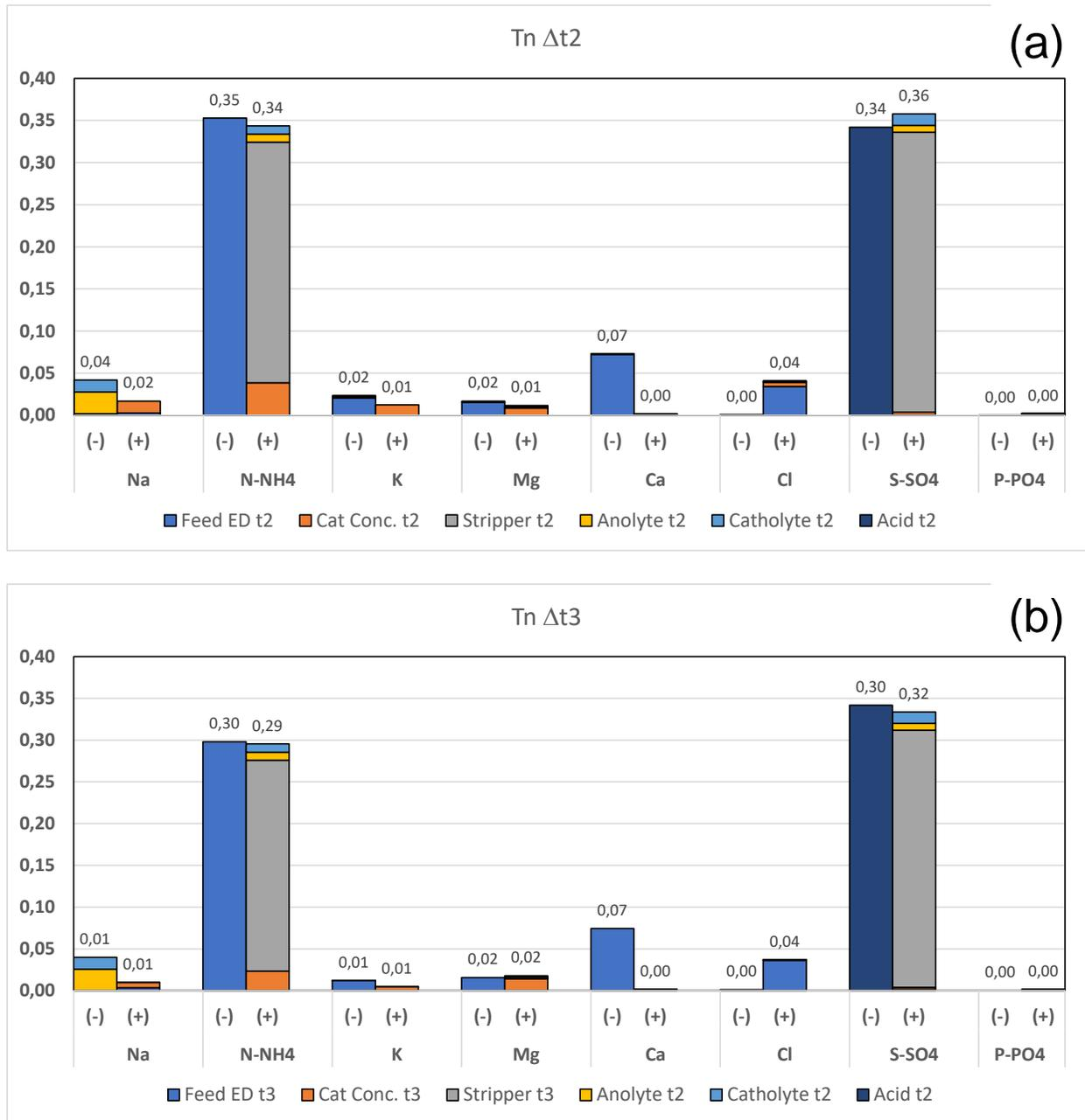
Figure 9. Transport number during  $\Delta t_2$  (a) and  $\Delta t_3$  (b).
