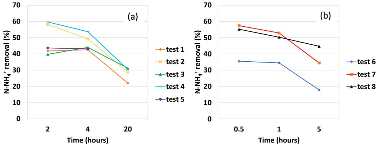
**Figure 5.**  $\text{NH}_4^+$  removal efficiency from the liquid digestate for Donnan tests (a) for continuous tests (b).
