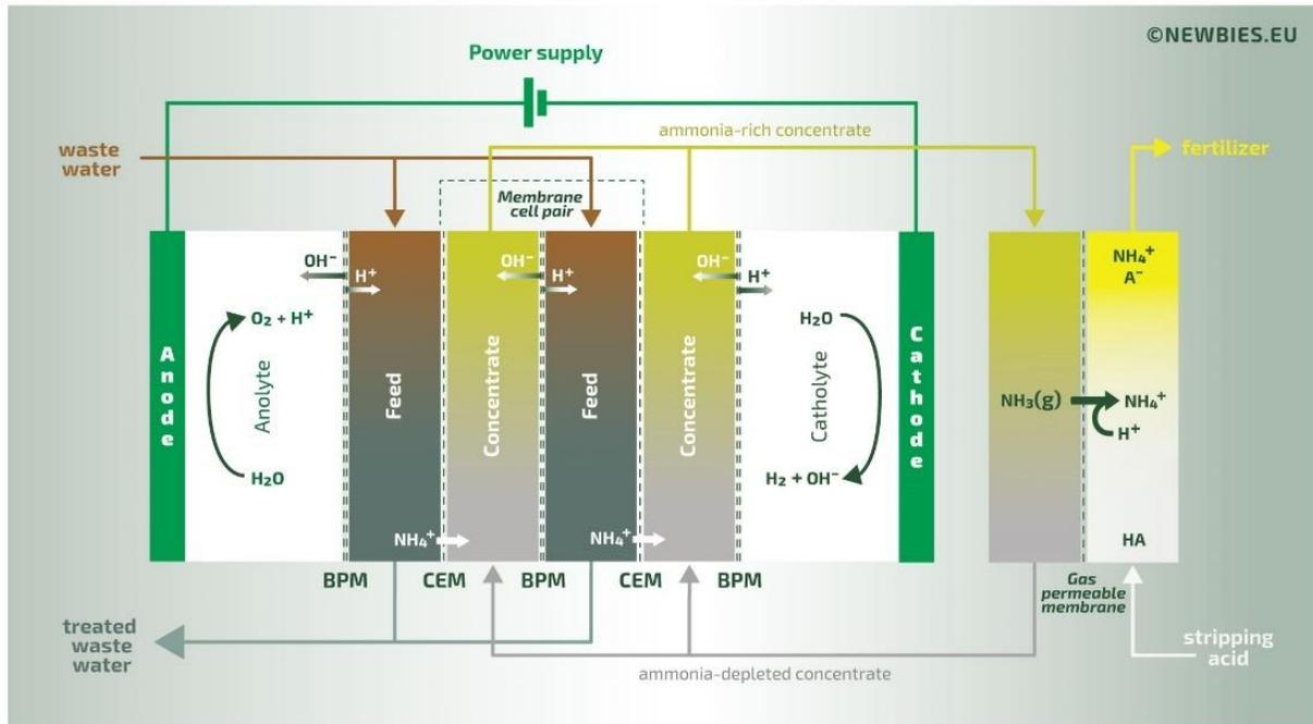
**Figure 1.** Concept flow diagram of the technology.
