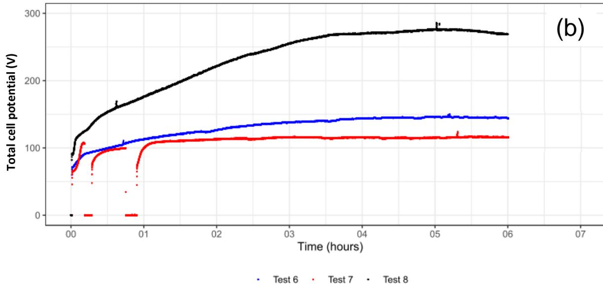
**Figure 6.** Average total cell potential per hour for the experiments run in Donnan mode (a) Total cell potential for the experiments run in continuous mode (b).
