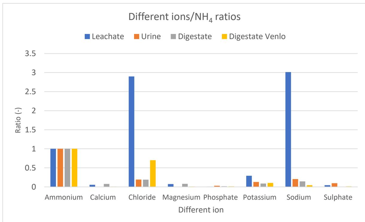
Figure 9 - Ratio of the different ions over  $\text{NH}_4^+$  content in the streams tested with the N.E.W.B.I.E.S pilot
