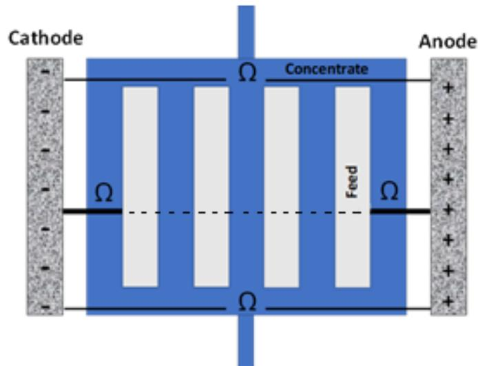
Figure 10 – Feed compartment filled with demi water acting as a good insulator, while concentrate compartment and cathode/anode filled with 0.250M  $\text{Na}_2\text{SO}_4$  act as good conductors.
