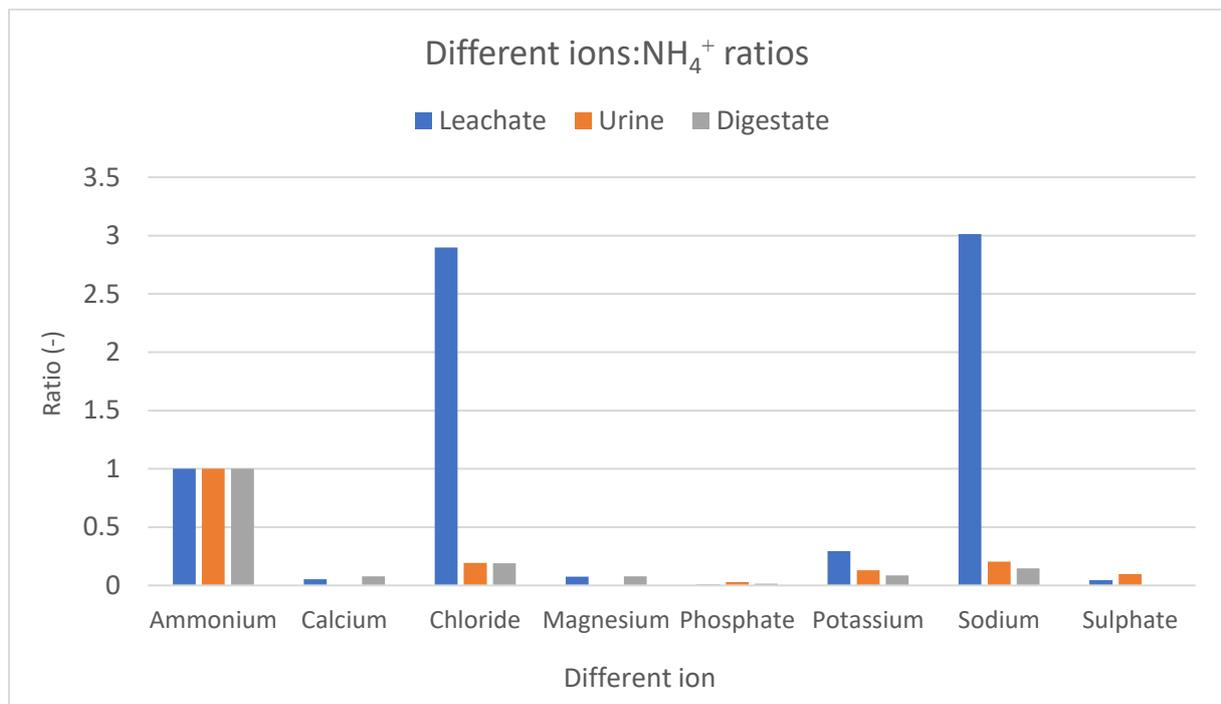
Figure 2: Ratio of the different ion over NH<sub>4</sub><sup>+</sup> concentration in the three streams tested with the N.E.W.B.I.E.S pilot
