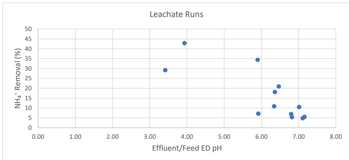
Figure 7: Feed pH effect to  $\text{NH}_4^+$  removal based on results with spider-stack
